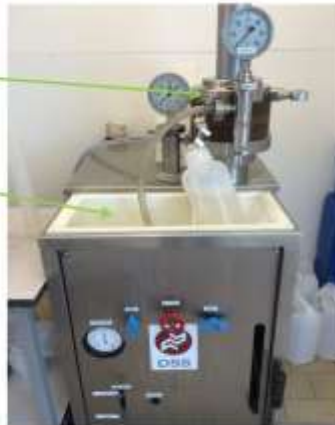
1- feed tank, 2 - valve, 3 - filter, 4 - high pressure pump, 5- valve for recirculation control, 6 - heat exchanger, 7 - manometers, 8 - membrane module, 9 - permeate outlet, 10 - pressure control
